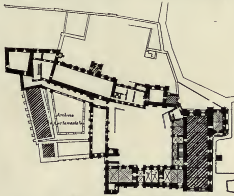
PLAN SHOWING PORTIONS OF THE PALACE OF THE POPES THAT HAVE BEEN OR ARE BEING RESTORED. (Darkly shaded parts restored.)
