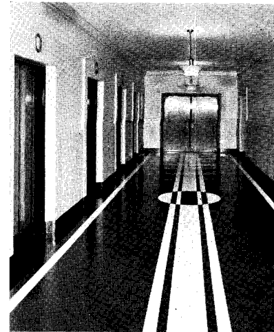
Elevator lobby, third floor, is 12 by 5 with a linoleum floor in terra cotta, and black. Base and dado are marble; and ceiling, plaster. Lighting is furnished 3 semi-indirect fixtures.
