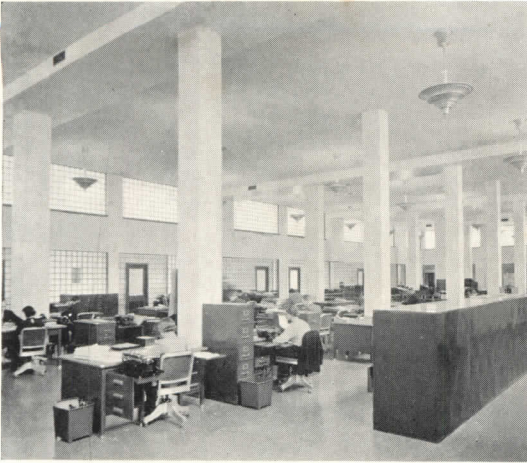
General office, second floor. Note that air-conditioning ducts are treated as ceiling beams.
