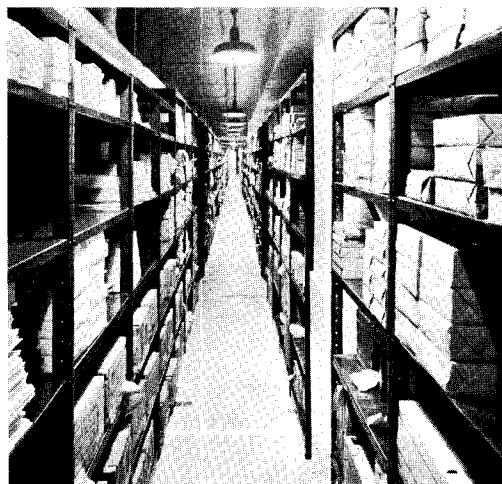
Basement supply space is equipped with 1,020 units of shelving in depths varying from 18 to 42 in. Shelving height is usually 8 ft. 3 in., sometimes 6 ft. 8 in. or 7 ft. 3 in. Lighting is of the direct type.
