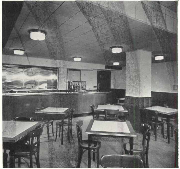
Coffee shop, or public dining space, in same hospital; note acoustic treatment of ceiling.
