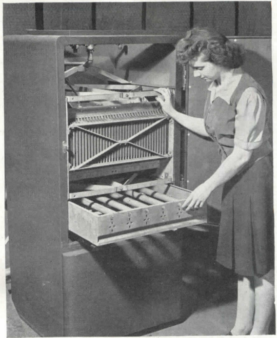
The electrostatic air cleaner (Precipitron) is being prepared for the home; photograph shows an experimental household model. Dust particles coming between grounded rods (diagram above) and high voltage wires, pick up a positive charge, pass on to dust collector, are attracted to and held by the negative plates
