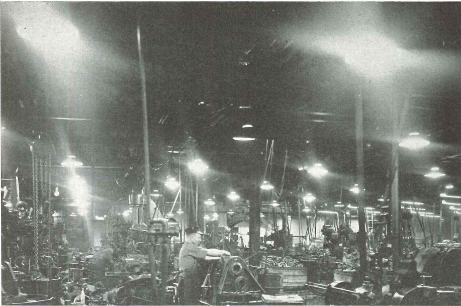
1. Illustrating some common defects of lighting: spottiness, shadows, dark ceilings and high contrast-ratios between fixtures and their background
