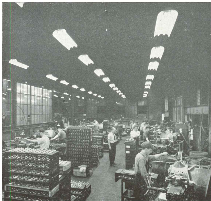
2. This is some better, but there is still too much contrast with the dark ceiling, even though fluorescent lamps are not as "bright" as filament lamps
