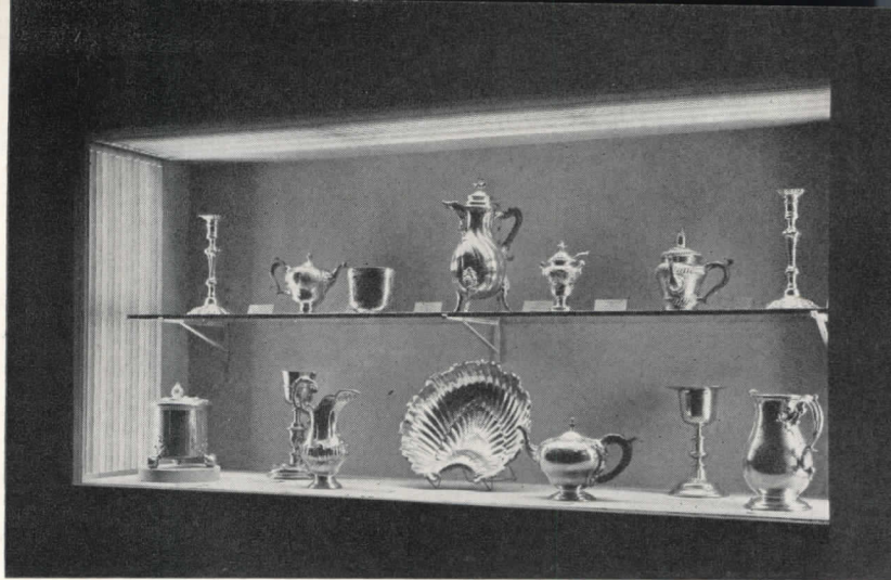
European silver in directionally louvered case; 100 f.c. of 4500° K. fluorescent light at center of deck, delivered from sides and top
