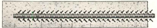
Laclede Multi-Rib Bars adequately transmit stresses to concrete by uniformly distributed anchorage. Small, closely spaced cracks do not open under load.
