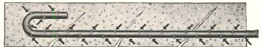
Old style reinforcing, with localized anchorage — conducive to widely spaced open cracks.
