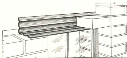
Pre-cut steel lintels save on-job labor
