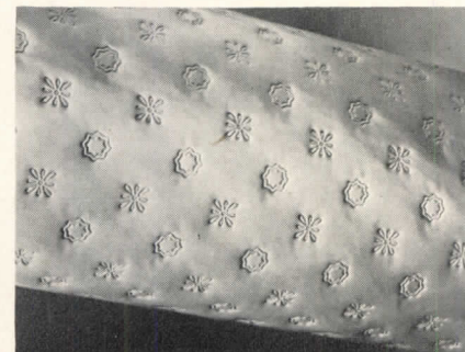
New process gives three-dimensional surface textures on plastic materials
