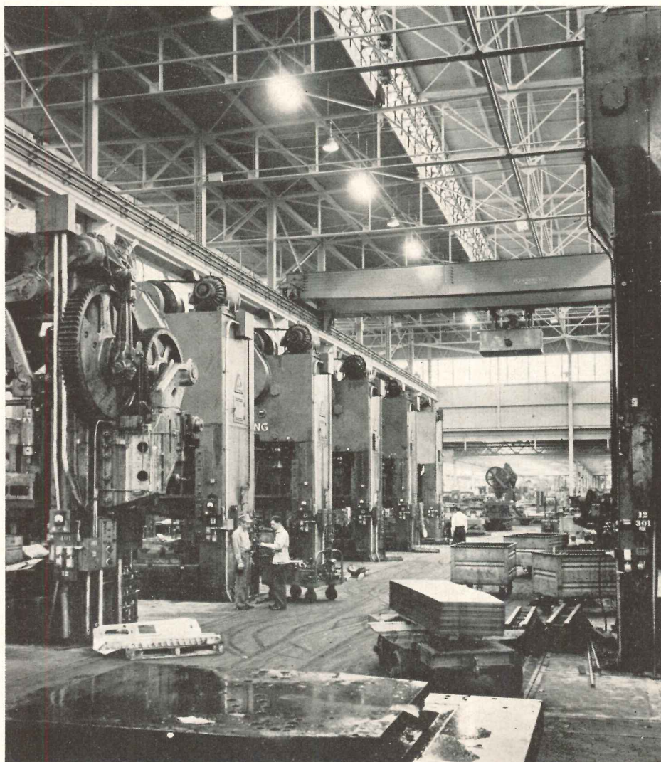
Photograph at left shows largest metal presses in line over pits. Photo above shows underneath view of press being serviced from the trench. Note floor section in place spanning pit trench between machines
