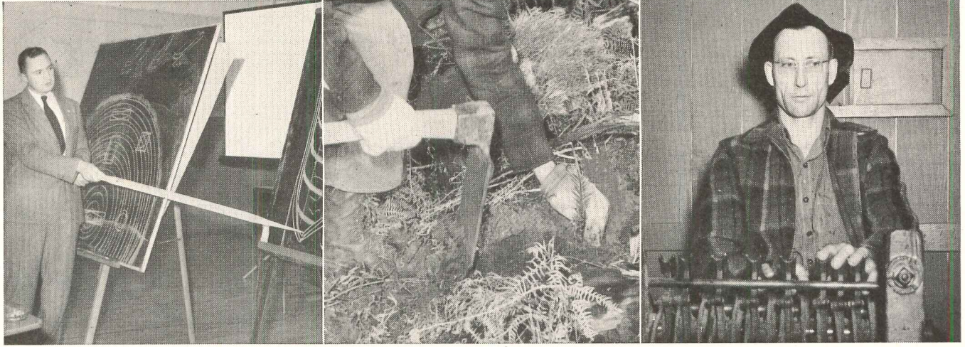
"PIANO PLAYER" this man is called. He operates a team of high speed saws, individually controlled from the "keyboard."
