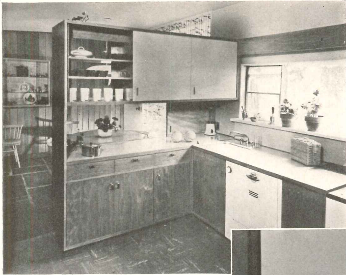
Kitchen (left) has pass-through to dining area beyond; birch shelves above can be opened from either side. Both kitchen and dining areas orient to southwest
