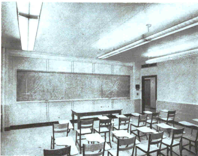
FIGURE 3: "Baker" school has 35db sound with lights on, room unoccupied. Over two people in room mask ballast "hum"
