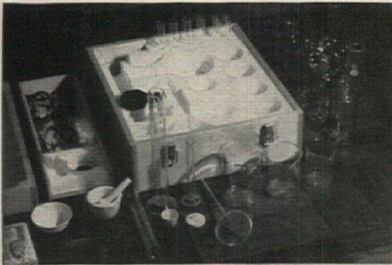
Left: To avoid need of various sizes of drawers at workbenches, students are provided with portable equipment containers stored in cabinets along the walls. Below: Four workbench arrangements show how components can be adapted to any of the science disciplines. Basic to all are the service/storage utility cabinets: (1) general chemistry; (2) organic and physical chemistry; (3) advanced physics (continuous work top); (4) biology, physics and zoology (center aisle aids supervision by laboratory instructor)
