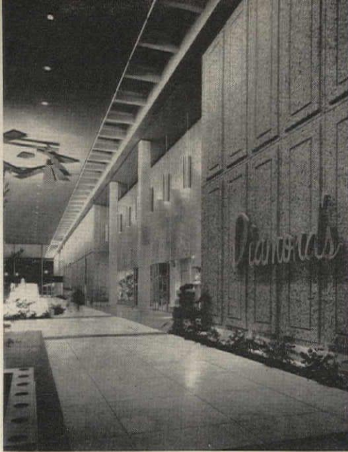
22-ft-high ceiling has clerestories on both sides. Two strips of concealed fluorescent fixtures bounce light off ceiling. Outer row of fixtures has aperture in top of light roof overhang. Small photo shows center mall during the day. Mall is punctuated by pools and illuminated fountains
