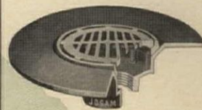
No. 7380-C "Super-Flo" Promenade Roof Drain with 4" wide deck flange and membrane clamping ring for use with Dex-O-Tex and similar roofing materials.
