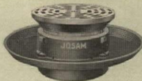
No. 300-A-SF Floor Drain with Super-Flo strainer for kitchen and shower areas. Greater strainer free area increases flow through drain. Perimeter slots permit water to keep drain clean.
