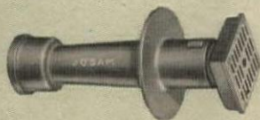
No. 0740-B Supply Fitting for swimming pools. V-port valve provides positive adjustment of flow into pool, square strainer to match tile, adjustable between body and face.
