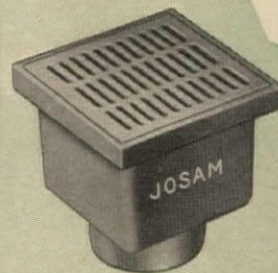
No. 5300 Floor Drain with square frame, tractor grate and sediment bucket for use in industrial plants to salvage materials discharged with waste water.
