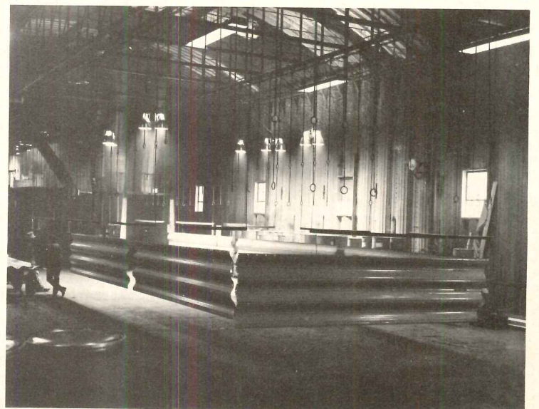
Galvanized steel panels pass through a multi-stage cleaning system and are primed before coating (top, left). Vertically reciprocating powder guns coat the panels and assure that all surfaces, including edges and joints, receive a uniform thickness (bottom, left). Coated panels are heated to 460 F in a tunnel oven so that vinyl powder melts and is fused to the substrate (top, right). Finally, panels are allowed to air cool (bottom, right).
