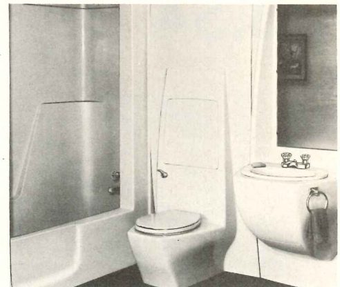
BATH SYSTEM / Now in development, the system is designed to provide a method of quickly plumbing and completing a 5 ft by 8 ft bathroom with three basic modules of fiberglass reinforced plastic. The units, when installed, complete two walls of the room with all plumbing concealed within the units, thus eliminating the need to pierce the wall or studs to install piping. Conventional vitreous china water closets and lavatory bowls are used with the system. ■ Wallace-Murray Corp., Eljer Plumbing-ware Div., Pittsburgh.
