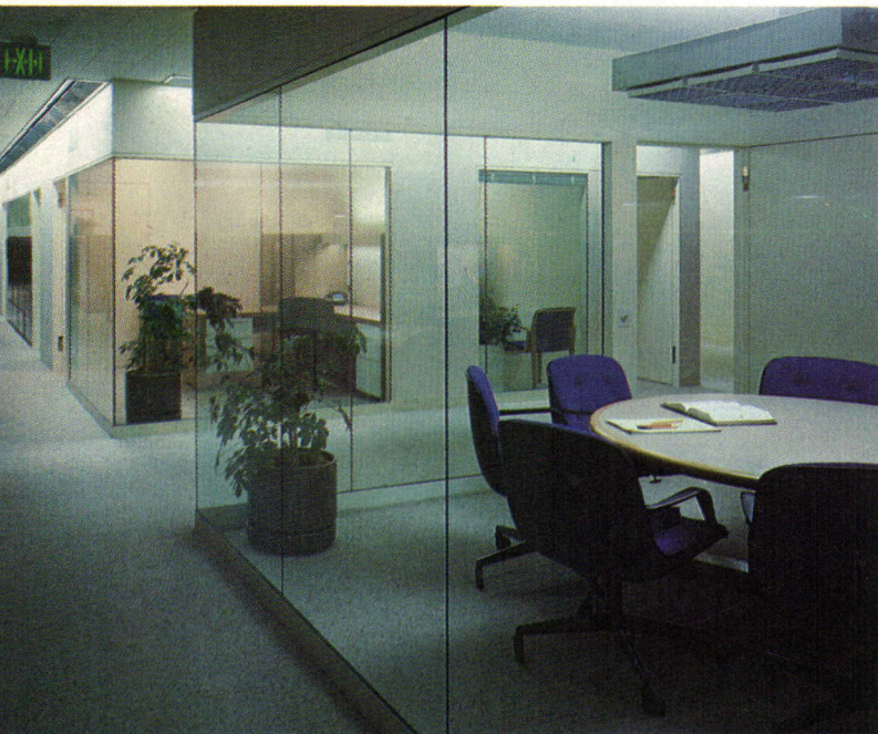
Illuminated surfaces provide ambient light and visual comfort, and give space definition and orientation. In private offices, a concealed uplight washes the ceilings evenly. All the core walls are washed by recessed fluorescent fixtures (lower left photo), while the glass walls of conference rooms (same photo) and the header of the executive secretary alcove (lower right) are not.
