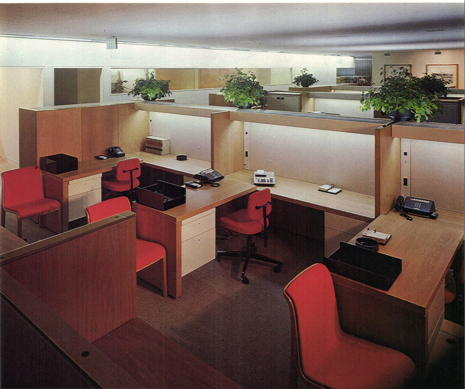
Work stations in the open-plan areas use Knoll-Stephens units that provide both task lighting and broad general uplight. A distributed file system separates the staff station from the corridor. One lighted core wall is shown in the left background. An opaque conference room wall (right background) displays photographs of the company's operations, illuminated by incandescent wall-washers.
