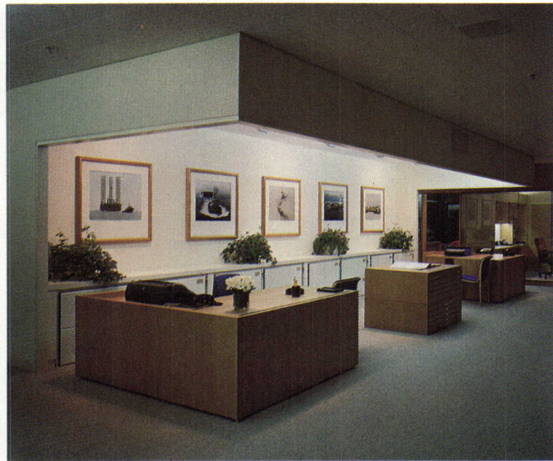
Illuminated surfaces provide ambient light and visual comfort, and give space definition and orientation. In private offices, a concealed uplight washes the ceilings evenly. All the core walls are washed by recessed fluorescent fixtures (lower left photo), while the glass walls of conference rooms (same photo) and the header of the executive secretary alcove (lower right) are not.
