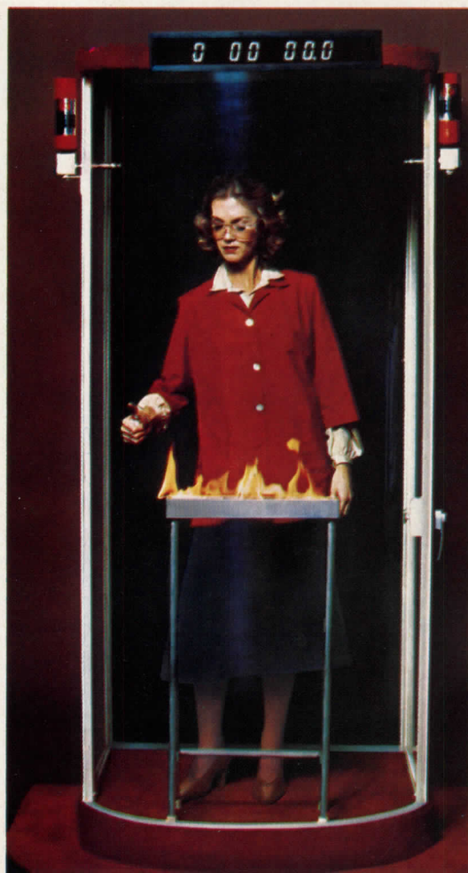
1. Flammable liquid ignited. Halon 1301 cylinders discharged.
