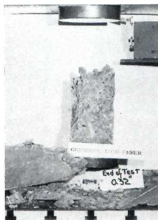
Plain concrete specimen simulating a building column ruptured at 0.32" compression when subjected to crushing loads. Considerable spalling occurred before failure.
