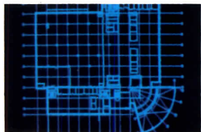
Structural grids created automatically.
