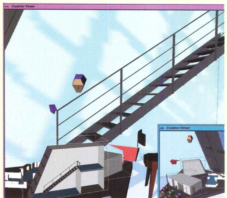
Face-like polygons denote the position of participants within the space. The small models on the table can be manipulated. A participant is shown slicing a section.
