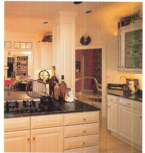
Black Alzak-cones in downlights (above) completely eliminate glare at the ceiling plane. A-19 lamps in open reflector downlights cover lots of horizontal space.
