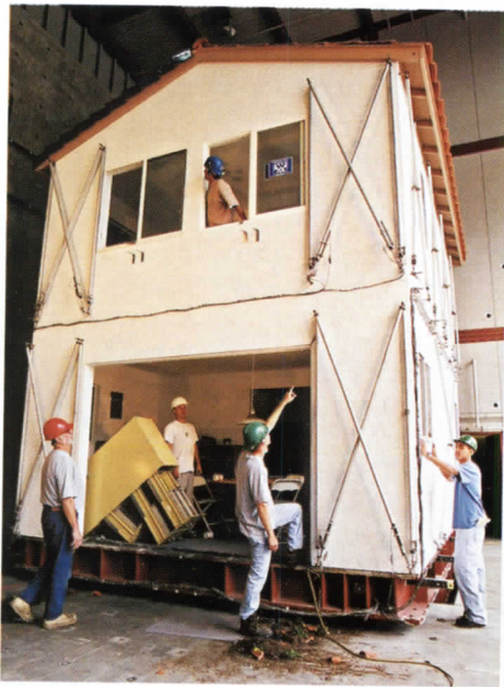
Researchers in San Diego placing a house on an earthquake simulator to measure its strength.
