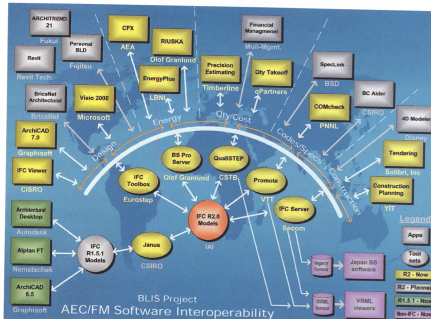
Building Life-cycle Interoperability Software (BLIS) demonstrates the ability of any IFC-compliant programs to operate on one another's building model data.
