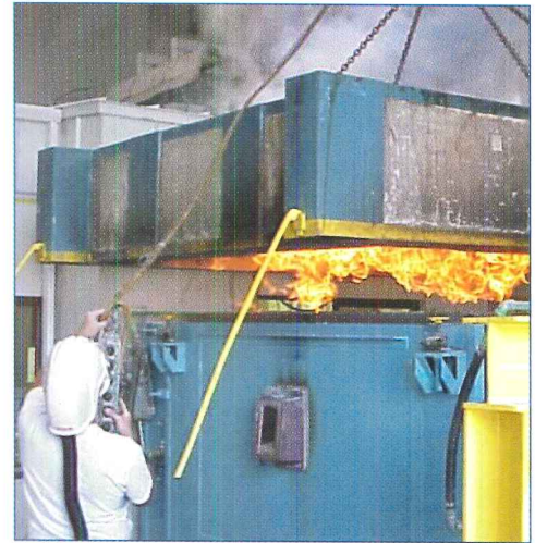
Fire testing is a critical performance criterion for wall, ceiling and floor assemblies. Here, a floor-ceiling assembly is removed from a testing furnace.
