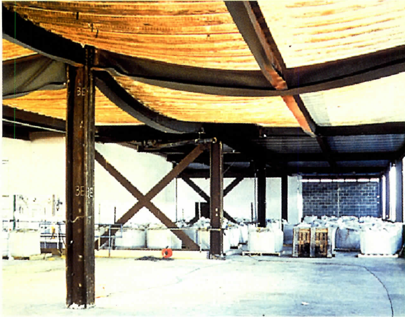
Beam in Cardington Tests after reaching temperature in excess of 1600° F.
