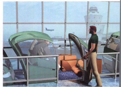
Taxi 2000's SkyWeb Express is a Personal Rapid Transit (PRT) system. Passengers select a destination, purchase a ticket, and enter a vehicle. Guideways take the cars directly to their destination without stopping.
