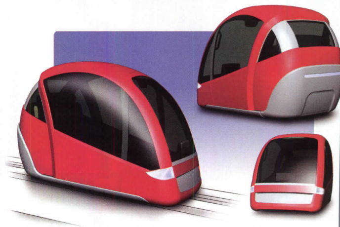
Taxi 2000's SkyWeb Express is a Personal Rapid Transit (PRT) system. Passengers select a destination, purchase a ticket, and enter a vehicle. Guideways take the cars directly to their destination without stopping.
