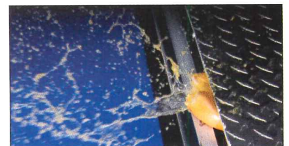
Actual demonstration of the closing force of a "lift assisted" non-Bilco floor door
