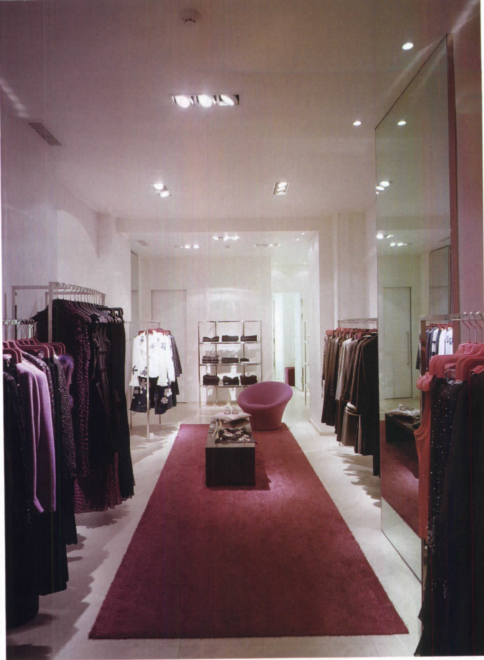
Recessed metal-halide lamps illuminate display areas for apparel and accessories (left). The juxtaposition of cascading crystal chandeliers and the high-tech pendants honors GUM's changing history (below).
