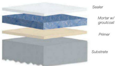
Configuration of decorative troweled mortar flooring.
