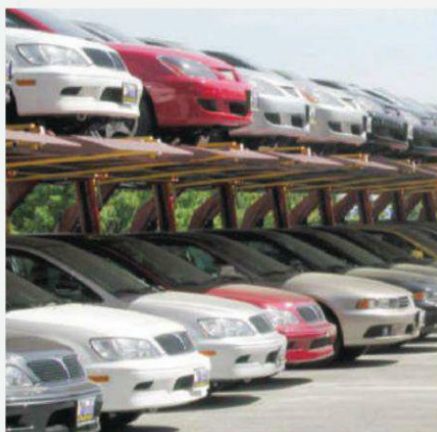
Left: Cantilever or "stacker" systems use hydraulics to park one car over another. These mechanisms require a trained valet driver to operate safely. Right: Four-post stackers use hydraulics to store up to five cars on top of each other. These mechanisms require a trained valet driver to operate safely.
