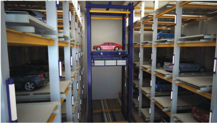
First-generation “mono-path” rolling hoist systems process transactions serially (one car at a time).
