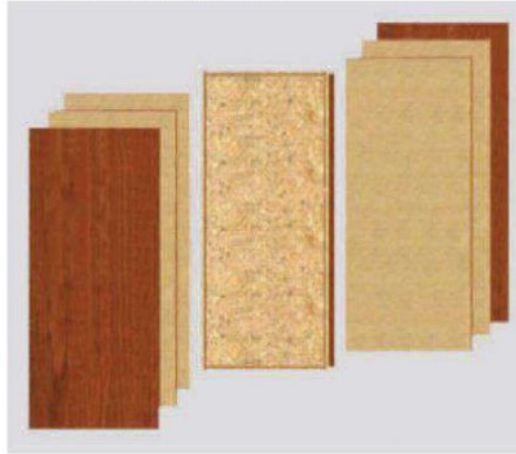
Commonly used for commercial applications, seven-ply wood doors include a core, backer materials, crossbands, and thinner face materials.
