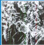
Xypex Crystallization (Initiated)
