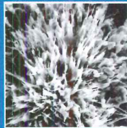
Xypex Crystallization (Mature)
