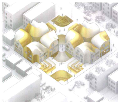
Bair's design for a residential block, as outlined in Cut/Fill , creates multiple corner-lot conditions and reorganizes building adjacencies.
