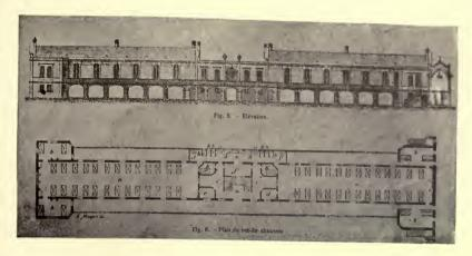
Fig. 24.—Hospital, Montpellier—Elevation of a Pavilion.
