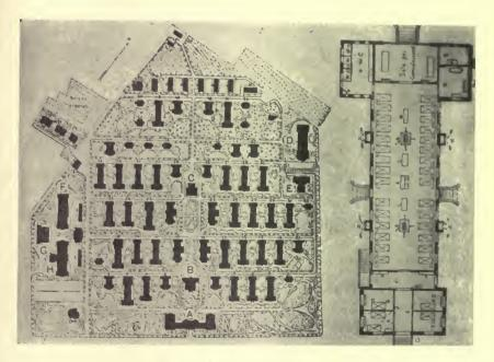
Figs. 15 and 15 a.- The New Hospital, Hamburg-Plan of a Pavilion.
