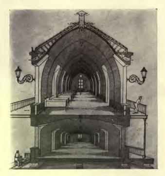
Fig. 23.-Hospital, Montpellier-Transverse Section of a Pavilion.
