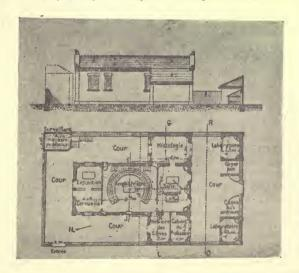
Fig. 26.—Hospital, Montpellier—Plan and Elevation of the Autopsy Pavilion.
