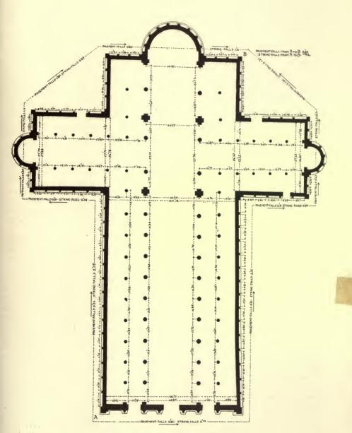
Fig. 5.—PLAN OF THE PISA CATHEDRAL. This plan includes the levels of the exterior pavement and string-courses and the curve of the south wall.
