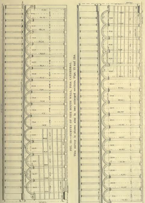
r-There are no surveys for the curve of the roof-line on the north wall, for which see photograph. Fig. FIG. 11.-SURVEY OF THE NORTH WALL, FISA CATHEDRAL.
