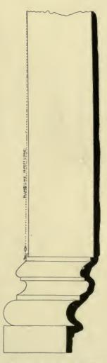
Fig. 20.—Block cut to a lean in the right portal of the facade of S. Michele, Pavia.
