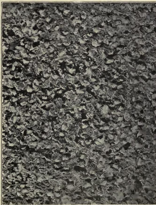
FIG. 10. SURFACE FINISHED BY PNEUMATIC HAMMER.
