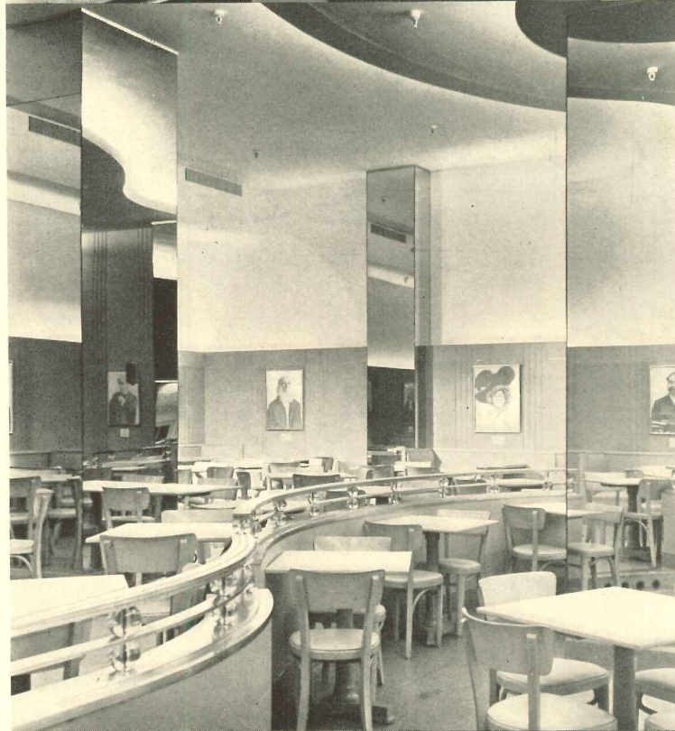
Interior, Longchamps Broadway Restaurant, New York City. Louis Allen Abramson, Winold Reiss Studios, Architects and Designers. Wall area above panels becomes reflecting surface for indirect lighting.
