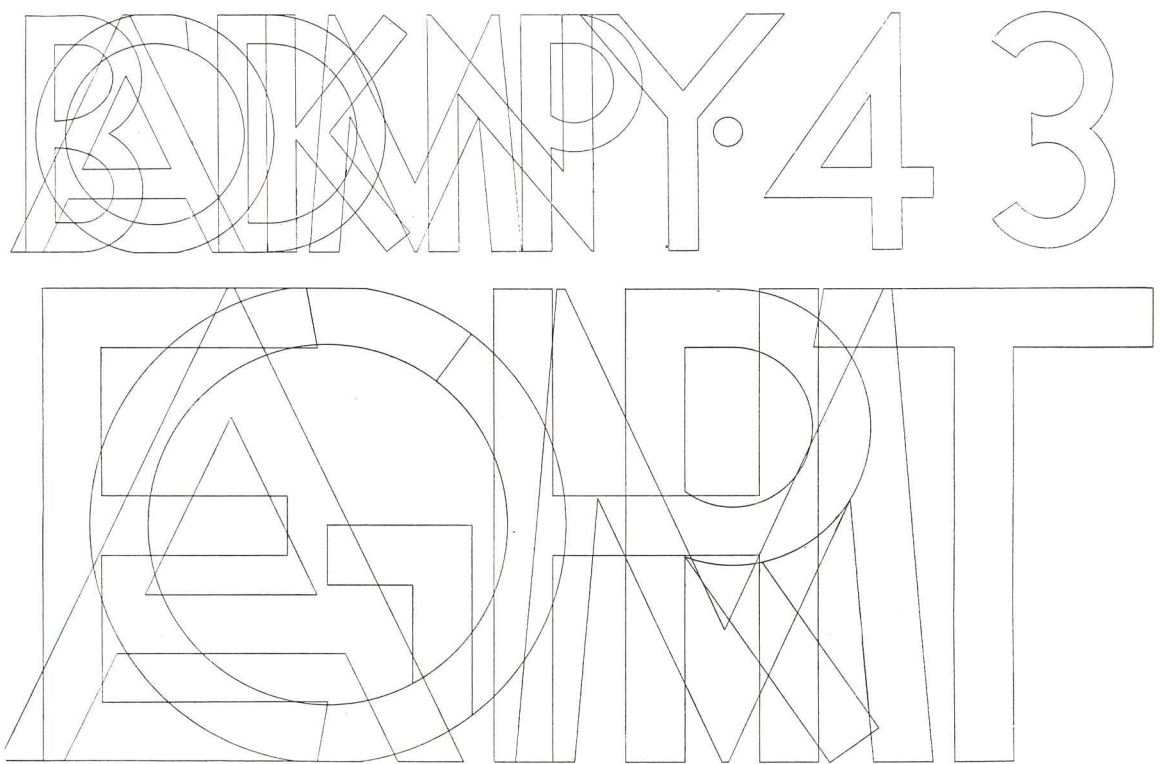
LETTERS for signs are drawn to full size combined on a small size sheet
