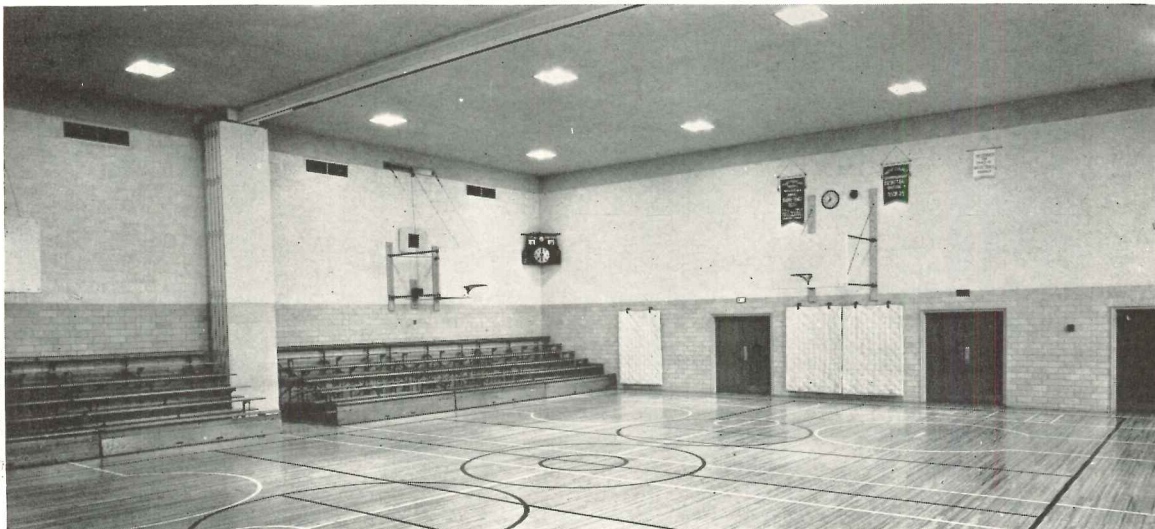
GYMNASIUM is convertible into two full gymnasia, one for boys, one for girls, by means of folding partitions
