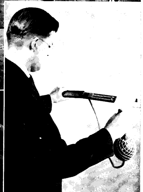
Taking Humidity Readings with Hand- Aspirated Psychrometer.
