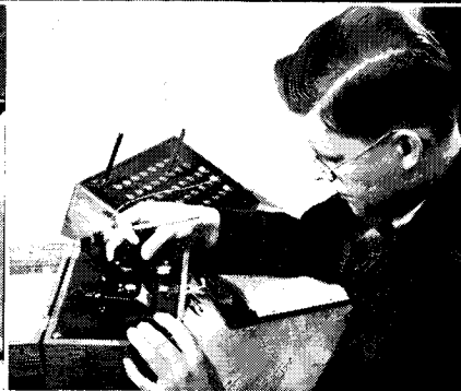
Taking Temperature Readings with Potentiometer at 43 Thermocouples.
