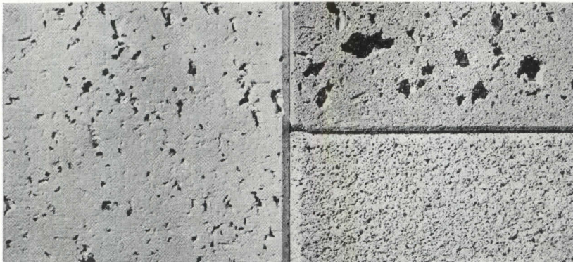
Left: Acoustone Type F, federal specification number VI; upper right: Muffletone, VI; lower right, Softone, VI
