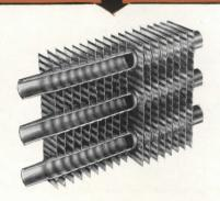
Ripple Fin coils mean better heat transfer because tubes are hydraulically expanded into fin collars locking them together in a permanent mechanical bond. Wide fin collars give greater area of metal-to-metal contact. Spun collar surfaces give smoother quality of contact.
