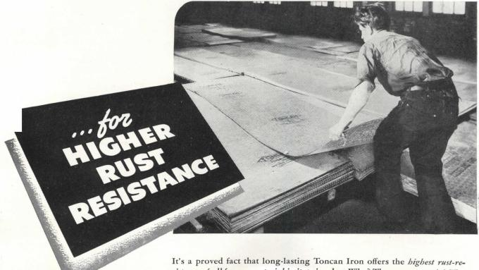
It's a proved fact that long-lasting Toncan Iron offers the highest rust-resistance of all ferrous material in its price class. Why? Three reasons: (1) The highly refined open-hearth iron, which is its basic ingredient. (2) Extra copper content—actually, twice that of copper-bearing steel and iron. (3) The addition of molybdenum, which multiplies the effectiveness of the alloyed copper.
