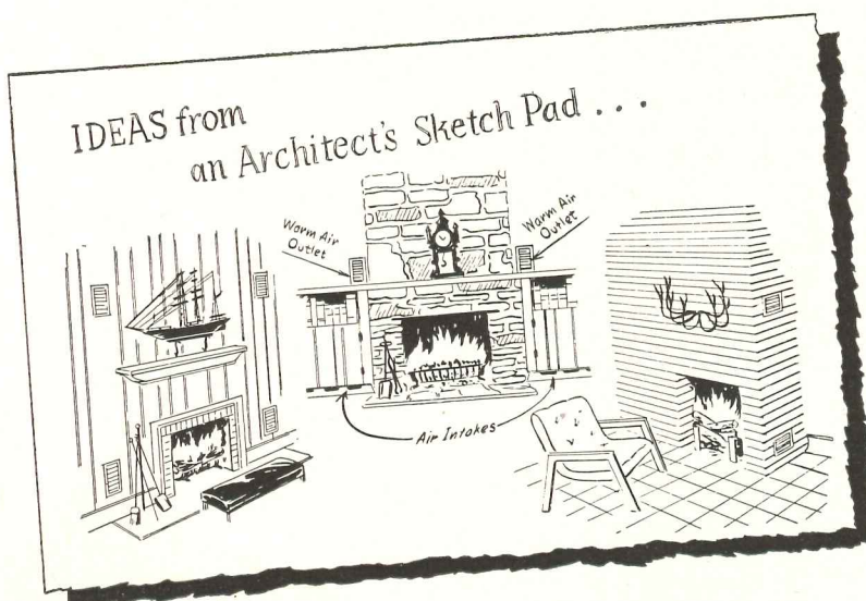
An example of warm air outlet grille placement in a fireplace with projecting mantel.
