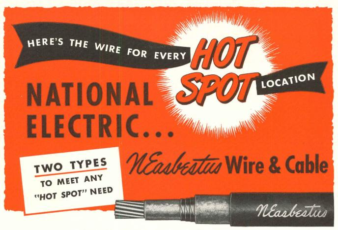
ASBESTOS-VARNISHED CAMBRIC—Recommended for conduit, raceway or open wiring in boiler rooms, steel mills, power plants, steam tunnels and factories where heat, moisture, corrosive fumes, oil and fire hazards are present. Sizes 18 AWG to 1,000 MCM. 600volt to 8000-volt ratings. Maximum operating temperatures up to 110° C. (230° F.) for 600-volt wire; up to 100° C. (212° F.) for 5000-volt wire.
