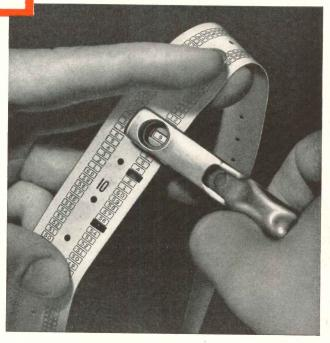
Other systems employing lugs, pins, cams, etc., are not only difficult to set up, but are subject to failure when pins drop out or break off.
