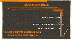
Information on ANACONDA Through-Wall Flashing and procedures for installation are detailed in Publication C-28. A copy will be forwarded upon request. Address The American Brass Company, Waterbury 20, Connecticut. In Canada: Anaconda American Brass Ltd.. New Toronto, Ont.
