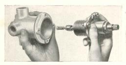
ONLY ONE MOVING PART—SIMPLICITY and durable construction insure many years of efficient carefree operation. Mixer body is made of bronze and parts subject to wear have a hard chromium finish.
