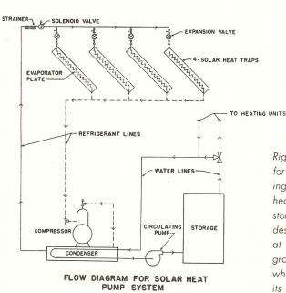
for sun-heated houses, showing variations in location for heat collectors and heat storage units, which were described by Prof. Anderson at the Symposium. Left: diagram of heat pump system which uses sun for part of its energy
