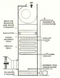
MIAGARA CONTROLLED HUMIDITY METHOD - FLOW DIAGRAM
