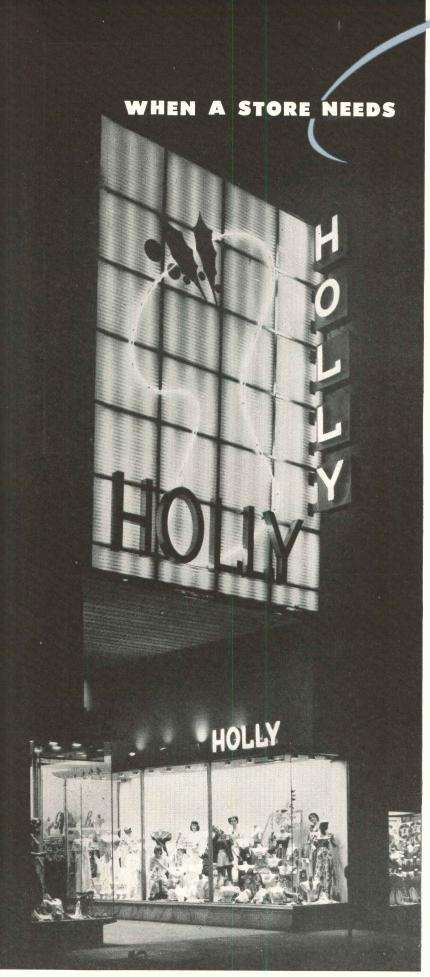
Designed by Morris Lapidus of New York, this 20-by-25-foot luminous store-front in Baton Rouge, La., was created by backlighting large panels of corrugated white translucent PLEXIGLAS. The interesting pattern is achieved by means of neon tubing behind the facade. Red and green PLEXIGLAS is used for holly leaves and berries mounted against the glowing acrylic background. Fabricated by Plastics Productions, Inc., New Orleans, La. Installed by Lamarr Advertising Agency, Baton Rouge, La.
