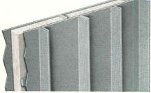
Wall No. 066 RIBBED EXTERIOR PLATES INTERIOR PLATES FLUSH
