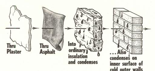
apor does not flow thru nor condense on outer or inner surfaces or reflective air spaces of multiple sheet accordion aluminum.
