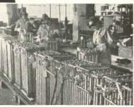
Attention to the many details that make up the completed unit typifies the Aerofin way. For instance, in this particular coil, careful brazing of the return tubes to the header plates assures leak-proof construction.
