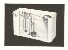
Interior view of Briggs Syphon Jet Closet Tank reveals latest design Anti-Syphon quiet operating flushing mechanism. This positive shut-off ballcock incorporates the latest type volume regulator, triple seal rubber ball, 1½-inch overflow tank valve, large refill tube and positive quiet action at high or low pressures. Every part quality engineered for lasting dependability.
