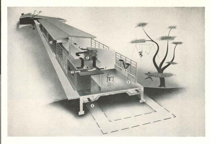
How the heating system operates: 1. Fresh air is taken in above exterior end door. 2. Air is drawn past steam heat coils by the fan. 3. Air leaves coils at 135F. 4. Air passes through concrete duct. 5. Air in duct keeps floor warm. 6. Air is thrown in front of cool glass area. 7. Half of air is recirculated (drawn from near ceiling). 8. Half of air is exhausted from classroom (drawn from near floor). 9. Air is exhausted to the outside
