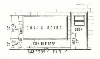
Typical classroom details. Above: section through washroom, with heights indicated for wainscoting, mirror and lavatory. Above right: heights of chalk board and door knob on typical wall elevation. Below right: arrangement of sink and wall cabinets
