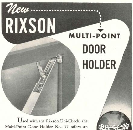
unsurpassed installation for doors which require several points of hold-open. Upon quick release by a slight manual opening of the door, it returns to closed position under control of the hydraulic checking device. Almost any number of positive hold-open points desired may be furnished.
