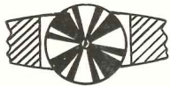
END VIEW OF CONCEALED BEARING SUPPORT Louver rotates on cylinder bearing points.
