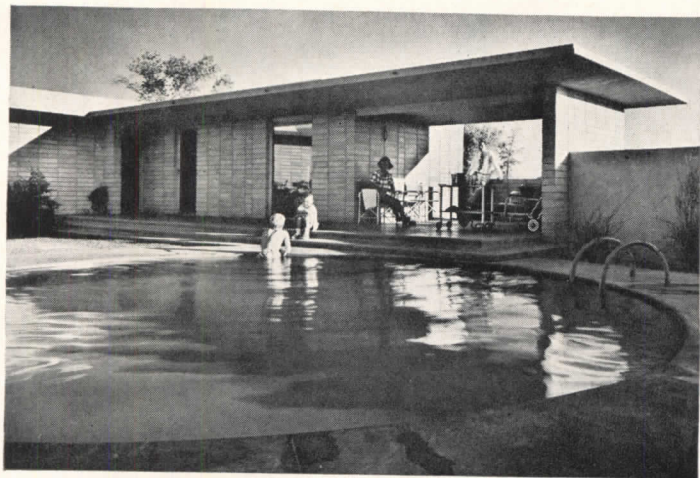
Above, left and right—Owen House, Phoenix, Ariz., Blaine Drake, architect Shelter at pool for sun protection—screening over terrace allows cool night air to descend to floor for after-dark comfort
