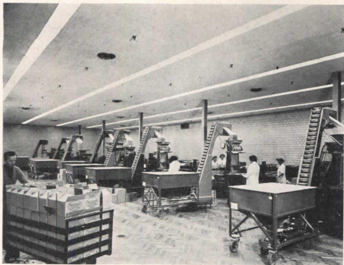
Above, packaging room; here tablets are automatically wrapped, packed in cartons and transferred to large finished products warehouse (photo below), where they are stored temporarily pending shipment
