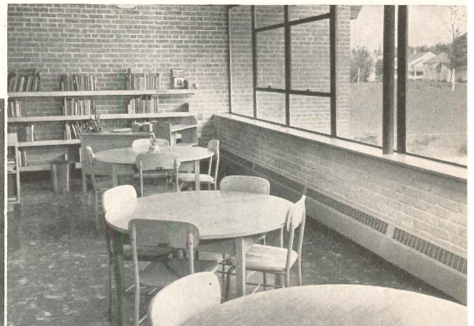
Left below: Teacher's lounge in Technical Building, Evanston Township High School, Evanston, Illinois. The exposed walls are heated with Webster Walvector painted to match wall color. Photo by Hedrich-Blessing.
