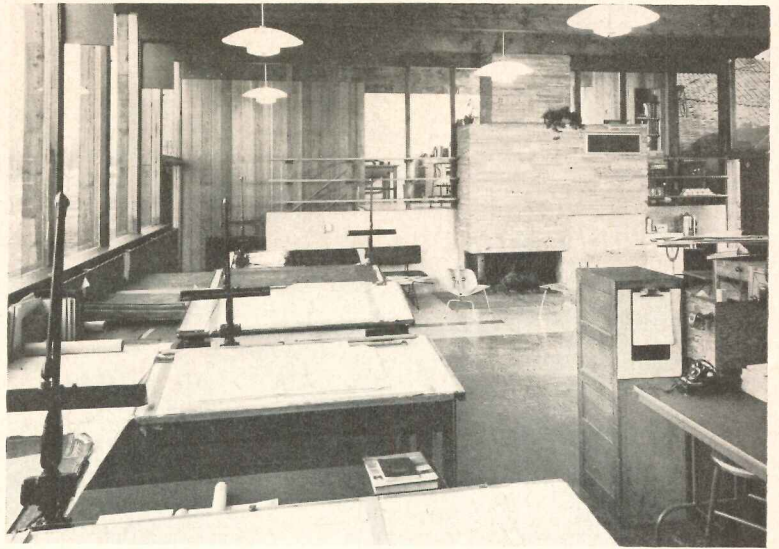
Drafting area of Jahr-Anderson has a 13-ft 6-in. ceiling with underside of roof deck exposed and finished natural. Rear wall is soft green with yellow flecks in vitreous cement over cinder block. Floor is light green asphalt tile. Lighting fixtures are concentric ring louver around silver bowl lamp with white translucent plastic domes, dramatizing natural wood ceiling
